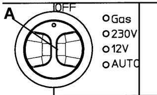
1. Set energy selector switch (A) to position "0" (OFF). The appliance is now fully switched off.
