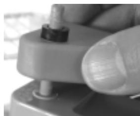
**6.** Position the hinge at the opposite side of the door and insert lower door.
