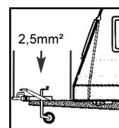
**The 12V circuit must be protected with a 16A fuse.**
