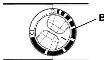
2. Use rotary switch (B) to regulate the temperature in the main refrigerator compartment.
