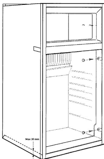
In the sidewalls of the refrigerator, there are four plastic sleeves with screws for securing the refrigerator. The sidewalls or rails attached for securing the refrigerator must be designed in such a way that the screws will remain firmly in place even when under increased load (while the vehicle is moving).
