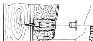
The screws must penetrate through the sheet metal casing of the refrigerator.
