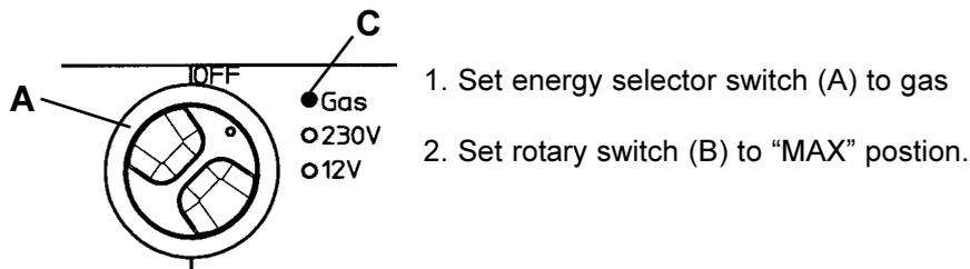
The ignition process is activated automatically, accompanied by a ticking sound approx. 30 sec. Upon successful ignition, the display LED (C) "Gas" lights yellow. The refrigerator is in function. Use rotary switch (B) to regulate the temperature in the main refrigerator compartment.
