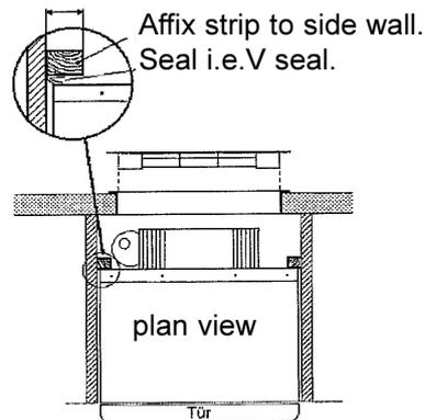
Stopper strips for example are affixed in the installation bay, at the sides, at the bottom and at the top and are fitted with flexible sealant strips
