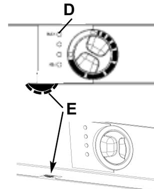
Underneath the fascia is a knurled knob for adjusting the brightness (see item E above)
