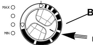
As shown, you are able to regulate the temperature of the cooling compartment, if necessary, by turning rotary knob (B).
