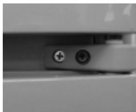
**3.** Unscrew middle hinge and remove lower door.
